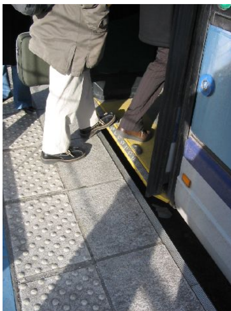
TEOR, level access and regular tram-type gaps thanks to guidance
