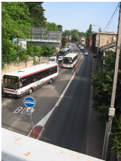
Lyon, exit from reversible reserved lane of the future C1 line, here authorised in the descending direction
