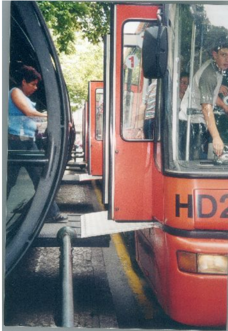
The efficient interface between the 24.5m bi-articulated bus and the tube station, platform height of about 70 cm Source Certu.
